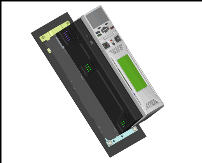
Figure 1-4 Locating the drive to the backplate
